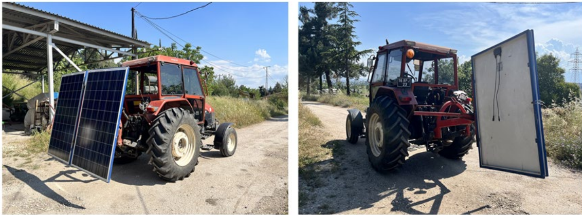
Figure 1 Three point hitched solar panel (work condition (left) and road condition (right)).
