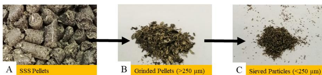
Fig 1. Preparation of sunflower seed shells (SSS) biomass pellets for thermogravimetric analysis
