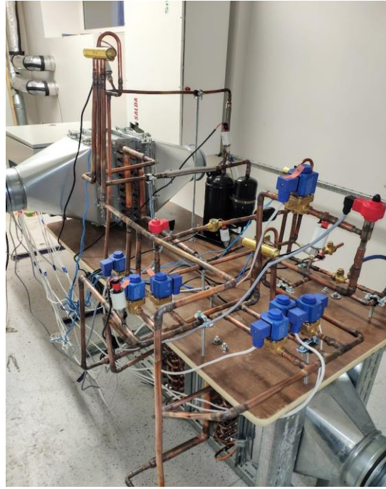
Fig. 4. Experimental stand of an HP for an AHU
