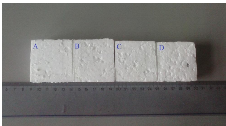
Fig. 3. Impact of vacuum: A – untreated polystyrene, B – after 10 min., C – after 20min., D – after 30 min.
