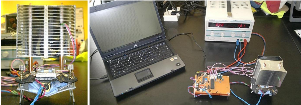
Fig. 5. Experimental laboratory setup for Peltier element performance measurements
