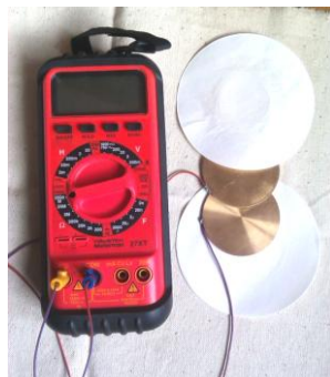
Fig. 3. “Wavetek Meterman 27XT” digital multimeter with two electrodes
