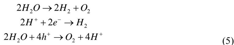
To provide these reactions in sunlight, material should absorb visible light. Most popular photocatalysts as  $TiO_2$  or  $ZnO$  absorb light only in the UV region. They can absorb only about 5% of sunlight, which greatly limits its practical applications. By now the main task in the science is to develop photocatalysts with enhanced visible light activity. From this point of view iron oxides stand out as promising materials for water splitting [6].
