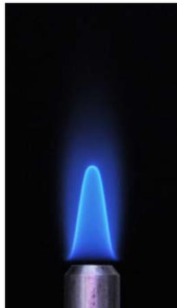
Fig. 3. The picture of illumination of the investigated rich premixed methane-air flame
